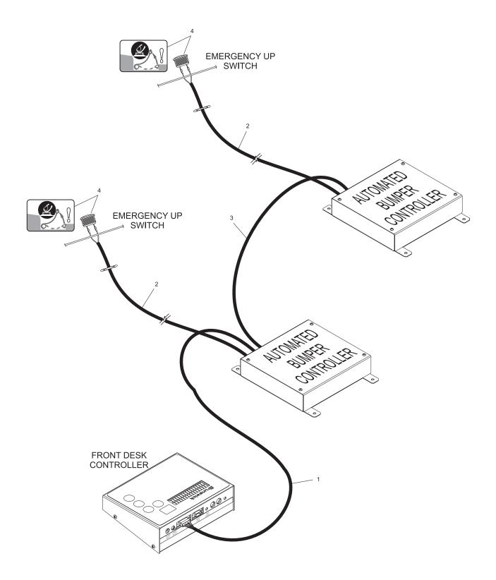
Automated Bumper System Cables Stand - Alone Configuration
